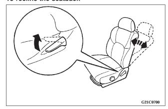
In order to recline the seatback, first lean your body forward slightly and pull the seatback lock lever up, and then lean backward to the desired position and release the lever. The seatback will lock in that position.
